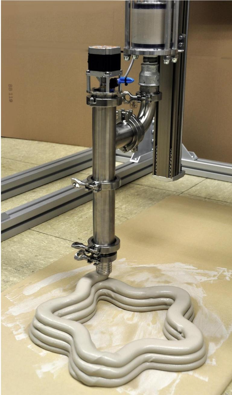
Large-scale mixing print head from stainless steel 304 with stepper motor Nema23 for mortar/concrete.
